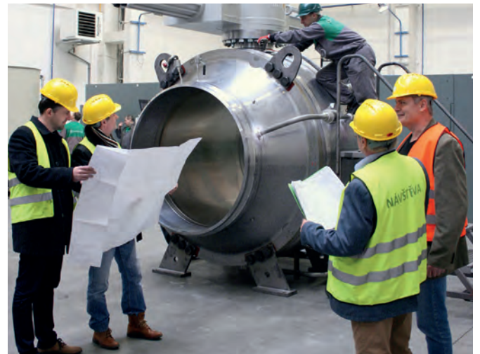
Inspection of ball valves DN 1400 AG for Eustream, Slovakia
