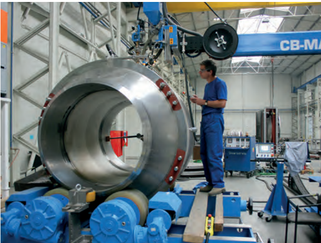
Automatic welding of ball valves DN 1400 AG
