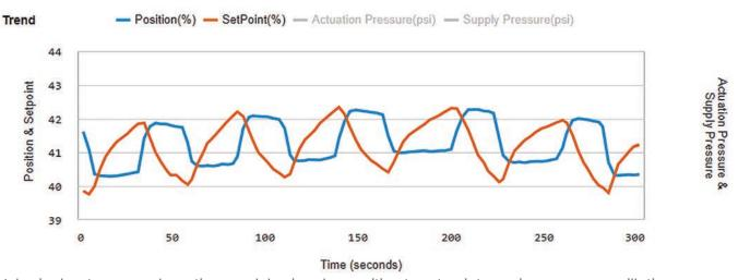
Valve is slow to respond, continuous delay is valve position to set point causing process oscillation.
