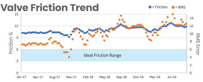
Packing friction consistently high over time, well above ideal range. Friction and RMS alerts have been constant over time, advising of stick-slip condition that will impact the valve responsiveness, resulting in control oscillation.
